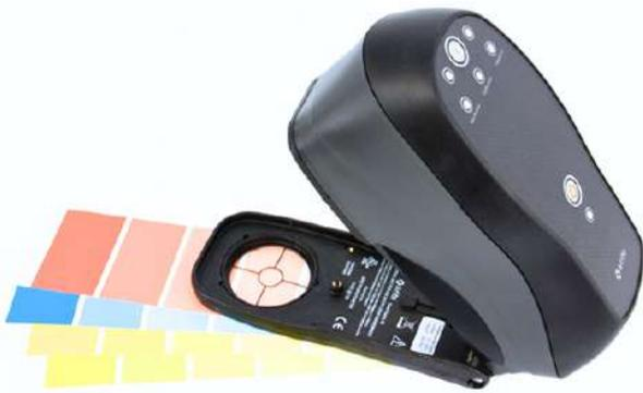
Looking for a fast, affordable quality control tool to monitor batch-to-batch variations and inconsistencies between customer specifications and production output? Need a way to speed up the creation and approval of samples? The Ci52 is a cable sphere spectrophotometer, affordable and versatile, for consistent measurement of color and appearance suitable for a wide range of materials, ideal for quality control applications.
